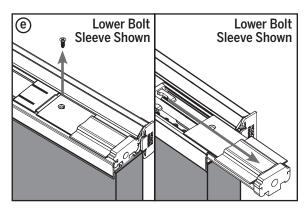
**e.** Remove the screw securing the lower bolt sleeve and slide the bolt sleeve out.
