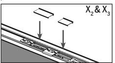
**Middle Trim Strips:** Align  $X_2$  with the bottom of the deadbolt plate and the top of the strike plate. Press down to secure. Align  $X_3$  with the bottom of the strike plate and the top of the flip lever assembly. Press down to secure.
