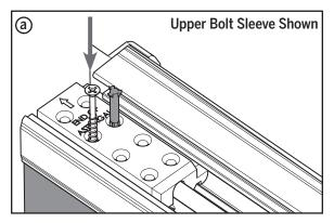
**a.** Keeping the orange securing pin in place on the upper bolt sleeve, install a #8 x 1-5/8" screw in the hole adjacent to the orange securing pin.
