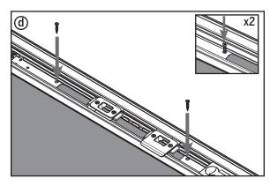
**d.** Install two  $\#8 \times 1$ " screws on either side of the cutout in the astragal body behind the strike and deadbolt plate.
