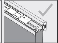
Ensure the upper and lower bolts are in the retracted position.
