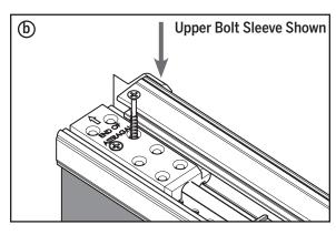
**b**. Remove the orange securing pin from the upper bolt sleeve and replace it with a #8 x 1-5/8" screw.
