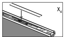
**Lower Trim Strip:** Align  $X_4$  with the bottom of the flip lever assembly and the top of the lower bolt. Press down to secure.
