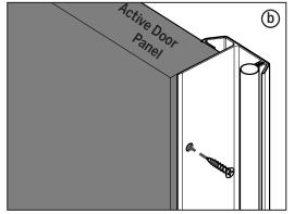
**b.** Insert the screws through the predrilled holes to secure the flange snug against the face of the active door.
