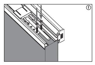
**f.** Install two #8 x 3"screws on either side of the bolt pin above the U-Shaped cutout in the astragal body. Predrill for the 3" screws with a 1/8" drill bit.
