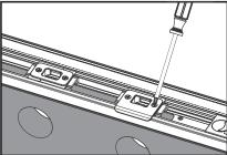
Secure the strike and deadbolt plates in their proper location by aligning them with the crossbore holes and tighten the screws into the retainers.
