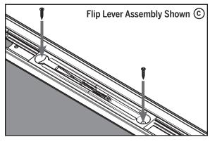
**c**. Install two #8 x 1" screws to secure the flip lever assembly into the door panel.
