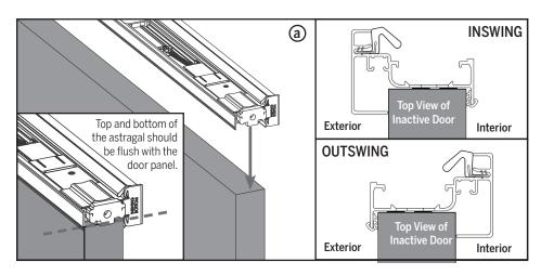
**a.** Place the astragal onto the door panel. For **Inswing** doors, the wide side of astragal goes on outside of the door. For **Outswing** doors, the wide side of astragal goes on inside of the door. The top and bottom of the astragal should be flush with the top and bottom of the door panel.
