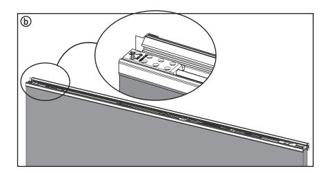
**b.** Press the astragal down along the length of the panel. An orange securing pin will pop up in the upper bolt sleeve. **Do not remove the pin at this time.**
