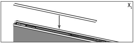
**Upper Trim Strip:** Align  $X_1$  with the top of the astragal and the top of the deadbolt plate. Press down to secure.
