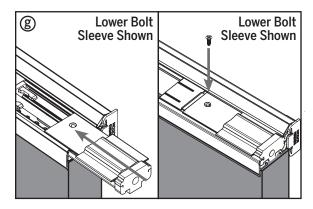
**g.** Return the bolt sleeve onto the lower bolt and reinstall the screw securing the bolt sleeve.
