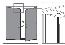
**c.** Close the inactive door panel. Ensure the weatherstrip forms a secure seal around the trim cap.
