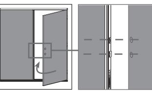
**b.** Close the active door panel and ensure the deadbolt and strike plates are aligned with the crossbore holes in the active door panel.
