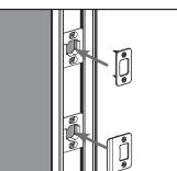
Cut Here **b.** Install the new hardware into the retainers by tightening the screws through the holes in the plates.
