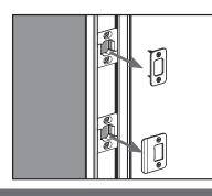
**a.** If installing new strike and deadbolt plates, remove the screws securing the old plates.
