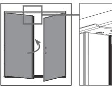
**a.** Close the inactive door. Make a mark at the location where the trim cap contacts the weatherstrip.
