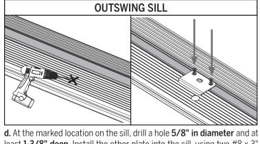
**d.** At the marked location on the sill, drill a hole **5/8**" **in diameter** and at least **1-3/8**" **deep.** Install the other plate into the sill, using two #8 x 3" screws.
