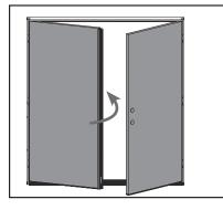
**a.** Close the inactive door panel until the weatherstrip on the header is compressed.
