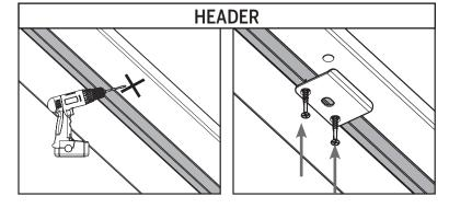
c. At the marked location on the header, drill a hole 3/8" in diameter and at least 1-3/8" deep. Install the header strike plate by screwing into the header, using two  $#8 \times 3"$  screws.
