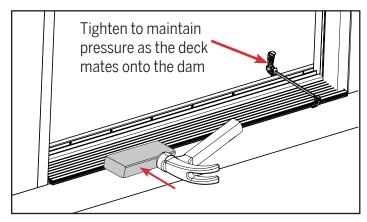
**e.** Returning to the initially connected side, use the block and hammer to connect the new sill deck to the substrate, moving evenly down the sill deck towards the clamp. Tighten the clamp as needed to maintain pressure and ensure the deck mates properly with the dam.
