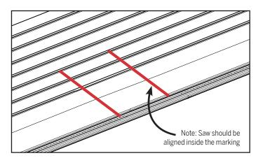
**f.** Once the marks are made, align the chop saw to the inside of markings on the sill and cut from the front of the sill deck to the break line in the sill.
