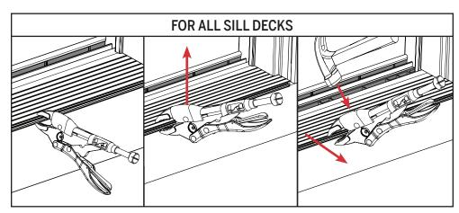
**c.** Once the aluminum deck is disengaged from the substrate, clamp vise grips onto the sill deck and lock them into place. While pulling the vise grips up and out, use a hammer to hit the vise grips away from the substrate. Repeat this along the length of the substrate. Set the removed deck aside to use as a template.
