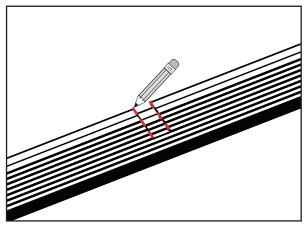
**d.** Using the old deck as a template, mark the notch location on the new deck.
