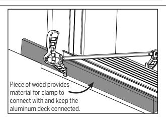
If flooring is installed and you cannot clamp behind the nosing: Position a piece of wood on the interor of the sill and attach the clamp to the back of the wood. This will provide a solid surface to use the clamp.
