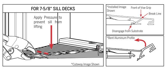
**b.** Clamp vise grips onto the sill deck 3"-6" from jamb, so the front of the vise grips are positioned just before the break line shown above. Bend the aluminum upwards to disengage it from the substrate. Apply pressure on the deck while bending upwards to prevent the sill from lifting and force the aluminum to bend. Repeat on the opposite end and along the length as needed.
