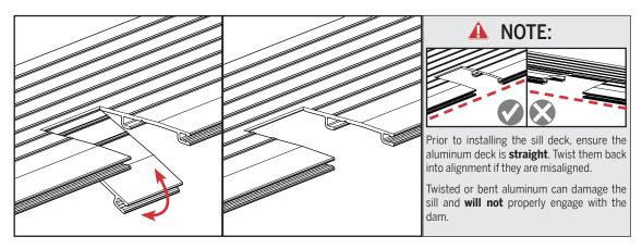
**g.** Once the two cuts are made, bend piece with hand along the break line to detach the cut piece of aluminum.
