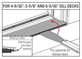
**a.** Use a stiff scraper to disengage the deck from the sill, starting at one end and moving along the length of the deck.
