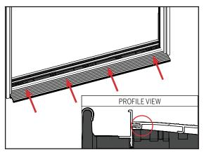
**b.** Slide the **new** aluminum deck evenly, as far as possible, onto the substrate.
