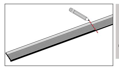
**b.** Mark the length of the old deck on the new deck. Use a chop or miter saw to cut down the new sill deck along that line.
