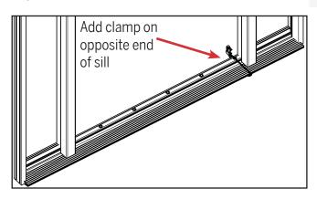
c. Use a wooden block and hammer to connect the new sill deck to the substrate on
