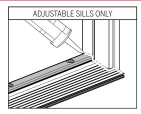
**b.** Adjust the cap to the appropriate height and caulk over the joint between the cap and jamb.
