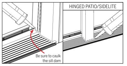
**f.** Apply an even bead of caulk around the jambs, including the dam. In a hinged patio or sidelite application, caulk the joint between the deck and mull.
