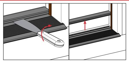
**a.** Rotate a stiff scraper under the dunnage cap to remove.
