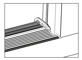
**a.** Use a putty knife or razor blade to remove the caulk seal along the jamb and mull if applicable. Use a flexible putty knife under the tenon to further break
