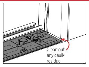
a. Clean out the tenon/jamb for any caulk residue.
