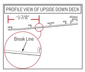
**e.** Identify the break line on the back of the sill deck.
