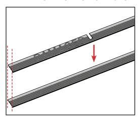
**c.** Once the new deck has been sized, align the new and old deck to mark the notch locations. Ensure both ends of the sill decks are aligned in order to mark the correct location.
