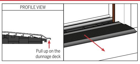
**b.** Once the dunnage cap is removed, pull up and out on the dunnage deck to remove.
