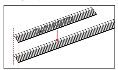
**a.** Align the removed deck onto the new deck to measure the correct length. If the deck is notched for a sidelite/hinged patio, use the notches to align the old and new decks.
