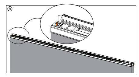
b. Press the astragal down along the length of the panel. An orange securing pin will pop up in the upper bolt sleeve. Do not remove the pin at this time. If present, ensure the backing of the tape is removed before pressing down.
