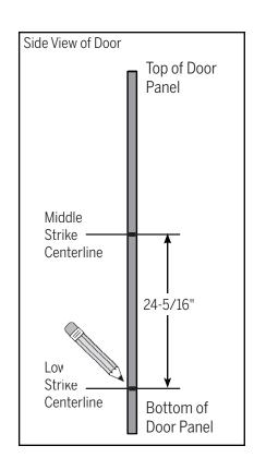
**c.** To determine the lower strike plate centerline, measure down 24-5/16"" from the middle strike centerline toward the bottom of the door and mark.
