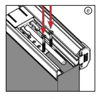
**e.** Install two #8 x 1" screw on the lower most hole next to the U-notch in the astragal body.
