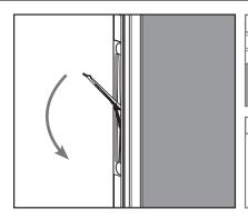
**b.** Engage the flip lever so the upper and lower bolt pins come in contact with the header and the sill. Mark these points of contact.
