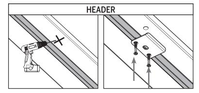
c. At the marked location on the header, drill a hole 3/8" in diameter and at least 1-3/8" deep. Install one of the strike plates into the header, using two #8 x 3" screws.
