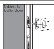
Cut Here **b.** At each location install new strike plates by screwing into the retainers.
