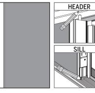
**b.** Engage the flip lever so the upper and lower bolt pins come in contact with the header and the sill. Mark these points of contact.
