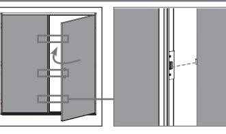
**b.** Close the active door panel and engage the lock to ensure the upper, middle and lower strike locations are properly engaged.
