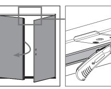
**b.** Open the inactive door. Using a utility knife, make a slit in the weatherstrip along the mark made.
