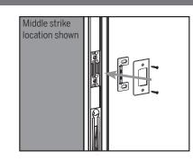
**b.** At each location install new strike plates by screwing into the retainers.
