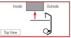
**a.** Position the security flange on the active door panel with the wide flange facing the outside of the house. Peel the tape backing and secure against the active panel.
