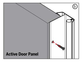
**b.** Insert the screws through the predrilled holes to secure the flange snug against the face of the active door.
