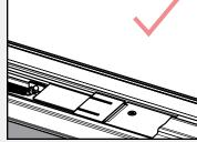
Ensure the upper and lower bolts are in the retracted position.
