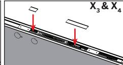
Middle Trim Strips: Install the X2 trim strip to be flush between the bottom of the upper strike plate and the top of the middle strike plate. Install the  $X_3$  trim strip to be flush between the bottom of the middle strike plate and the top of the flip lever assembly. Install the  $\mathbf{X_4}$  trim strip to be flush with the bottom of the flip lever assembly and the top of the lower strike plate.
