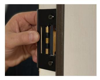
If adjustment of the strike is required to either loosen or tighten fit with weatherstrip, first partially loosen short screws.
