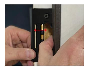
While holding top strike plate in position, move lower reinforcing plate assembly to the left or right – as needed to loosen or tighten door panel fit.
