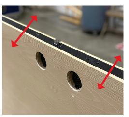
Check to confirm proper placement of the lock. Ensure entire length lock face plate is flush with edge face of panel. If lock does not sit flush, remove lock and check for debris in pocket. It may be necessary to verify mortise pocket dimensions if no debris or contamination is present.
