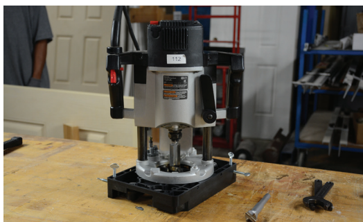
A plunge base router (1/2" Collet & 2-7/8" Minimum Plunge Depth)
