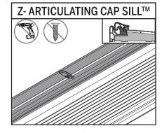
**NOTE:** If using a Z-AC sill, **no drilling is necessary** as the bolt receiver is preinstalled.
