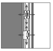
**c.** If it is not aligned, loosen screws and slightly adjust the locations of the plates.
