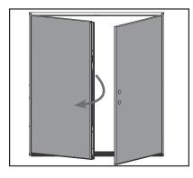
**a.** Close the inactive door panel until the weatherstrip on the header is compressed.
