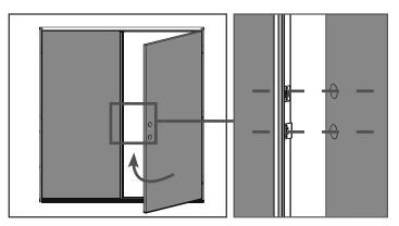
**b.** Close the active door panel ensure the deadbolt and strike plates are aligned with the crossbores on the active door panel.
