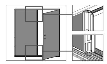
**a.** With the inactive door panel closed, engage both the upper and lower bolts to ensure they fit into the bolt receivers smoothly.
