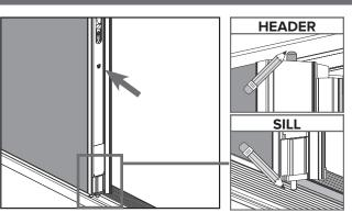
**b.** Press and engage the upper and lower bolts so the bolt pins come in contact with the header and the sill. Mark these points of contact.
