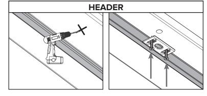
**c.** At the marked location on the header, drill a hole **3/8" in diameter** and at least **1-3/8" deep.** Install the header strike plate into the header using two # $6 \times 1-1/2$ " screws.
