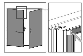
**a.** Close the inactive door. Make a mark at the location where the trim cap contacts the weatherstrip.
