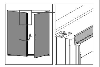
**c.** Close the inactive door panel and ensure the weatherstrip forms a secure seal around the trim cap.
