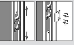
**d.** Adjust the location of the two pieces of the retainer and install the new hardware.
