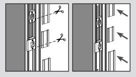
**e.** Resize the trim strip to fit flush against the deadbolt and strike plates and install into the astragal.
