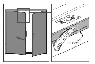
**b.** Open the inactive door. Using a utility knife, make a slit in the weatherstrip along the mark made.
