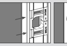
**a.** Remove the retainers from the astragal body by pushing the tabs in and rotating the retainer out.
