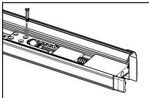
**a.** Return the lower bolt or the lower bolt sleeve removed in Step 1 by sliding back into the astragal . Return the orange securing pin or the screw.
