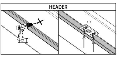
**b.** At the marked location on the header, drill a hole 3/8" in diameter and at least 1-3/8" deep. Install the upper strike plate by screwing into the header.
