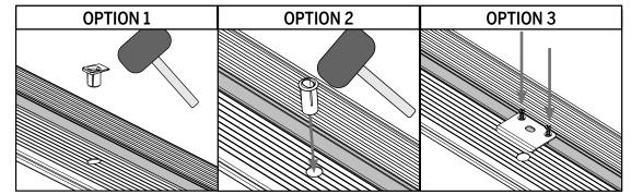
**d.** At the drilled location, install the sill receiver cup or sill strike plate based on the astragal type.
