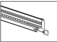
**a.** Install the finned trim cap on the wide side of the astragal and reinstall the tail cap removed in Step 2 on the narrow end if it was present.
