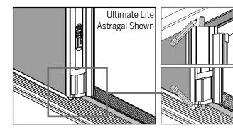
**a.** Press and engage the upper and lower bolts so the bolt pins come in contact with the header and the sill. Mark these points of contact.
