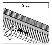
**c.** At the marked location on the sill, drill a hole **5/8" in diameter** and at least **1-3/8" deep.**
