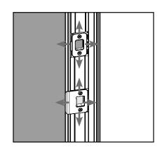
**c.** If the plates are not aligned correctly, loosen screws and slightly adjust the locations of the plates.
