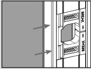
**a.** Remove the retainers from the astragal body by pushing the tabs in and rotating the retainer out.
