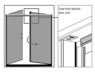
**c.** Close the active door panel and ensure the weatherstrip forms a secure seal around the trim cap.
