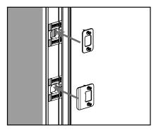
**b.** Install the strike and deadbolt plates by screwing into the retainers.
