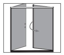
**a.** Close the inactive door panel until the weatherstrip on the header is compressed.
