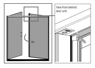
**a.** Close the inactive door. Make a mark at the location where the trim cap contacts the weatherstrip.
