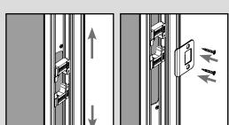
**c.** Break retainer in half using the bend lines. Return the two pieces of the retainer to the astragal and adjust to fit the larger hardware.
