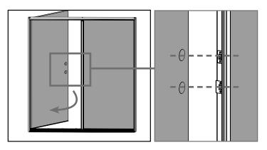
**b.** Close the active door panel and ensure the deadbolt and strike plates are aligned with the crossbores on the active door panel.
