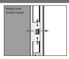
**c.** If the plates are not aligned correctly, loosen screws and slightly adjust the locations of the plates.
