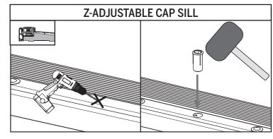
**d.** At the marked location on the sill, drill a hole **5/8" in diameter** and at least **1-3/8" deep.** Install the lower bolt receiver by tapping into the sill using a rubber mallet.
