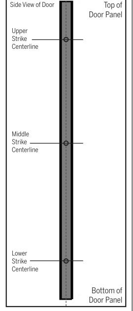
**f.** Using a 1" spade bit, drill a 1/2" deep hole at each center point. Clear debris from the holes.
