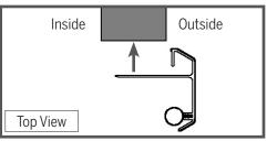
**a.** Position the security flange on the active door panel with the wide flange facing the outside of the house. Peel the tape backing and secure against the active panel.
