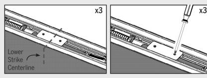
Adjust the location of the strike plates based on the three strike centerlines marked in Part A ( Page 2). Tighten the screws to secure them into place.
