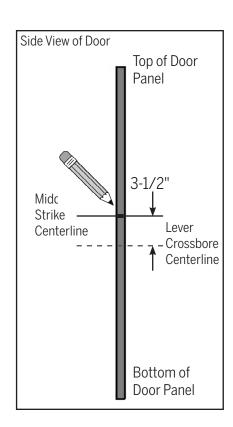
**b.** To determine the middle strike plate centerline, measure 3-1/2" up from the lever crossbore centerline towards the top of the panel and mark.
