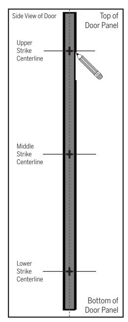
**e.** Determine the center point on the upper, middle and lower strike centerlines and mark the locations.
