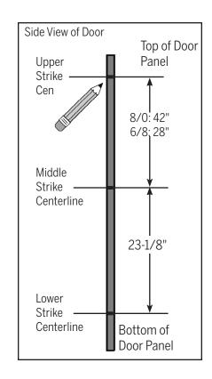
**d.** To determine the upper strike plate centerline, measure from the middle strike centerline up 28" for 6/8 doors or 42" for 8/0 doors and mark.
