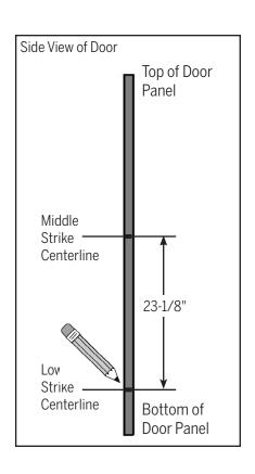
**c.** To determine the lower strike plate centerline, measure down 23-1/8" from the middle strike centerline toward the bottom of the door and mark.
