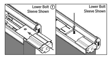
**f.** Return the bolt sleeve onto the lower bolt and reinstall the screw securing the bolt sleeve.
