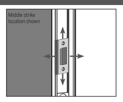
**c.** If the plates are not aligned correctly, loosen screws and slightly adjust the locations of the plates.
