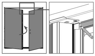
**a.** Close the inactive door. Make a mark at the location where the trim cap contacts the weatherstrip.
