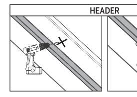
**c.** At the marked location on the header, drill a hole **3/8" in diameter** and at least **1-3/8" deep.** Install one of the strike plates into the header, using two #8 x 3" screws.
