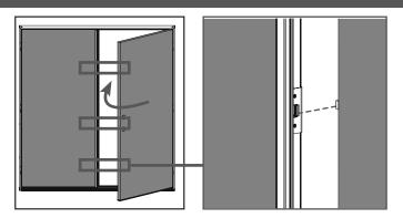
**b.** Close the active door panel and engage the lock to ensure the upper, middle and lower strike locations are properly engaged.
