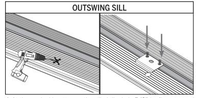
**d.** At the marked location on the sill, drill a hole 5/8" in diameter and at least 1-3/8" deep. Install the other strike plate into the sill, using two  $\#8 \times 3$ " screws.
