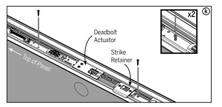
**k.** Install two #8 x 1" screws into the holes in the astragal body on either side of the strike retainer and deadbolt actuator.
