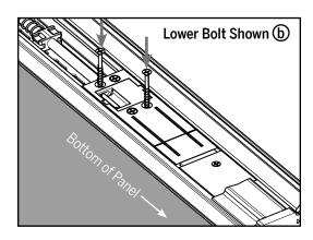
**b.** Remove the orange securing pins from the lower bolt and replace them with #8 x 1-1/2" screws.
