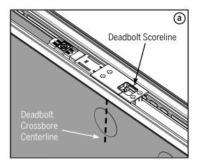
a. Check where the deadbolt actuator scoreline is positioned relative to the deadbolt centerline.
