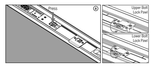
**a.** Operate the deadbolt actuator by pressing down on it. Ensure the top and bottom lock pawls move between engaged and disengaged positions.
