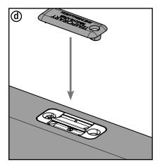
**d.** Reinstall the spacer into the keeper assembly.
