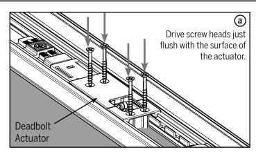
a. Drill Ø1/8" x 1-1/2" deep pilot holes at each deadbolt actuator hole. Install four #8 x 3" painted screws into each actuator hole.
