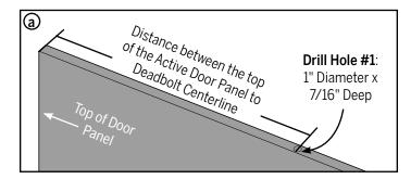
**a.** Mark the center of the rout location at the centerline of the deadbolt crossbore. Once marked, drill a hole that is 1" in diameter and 7/16" deep.
