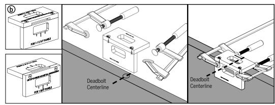
**b.** Position the deadbolt centerline to be lined up with the lower small mark on the template. Make sure to use the side of the template that matches the door panel thickness.
