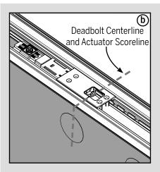
**b.** If the actuator scoreline is in line with the panel deadbolt crossbore centerline, skip to Step 9.
