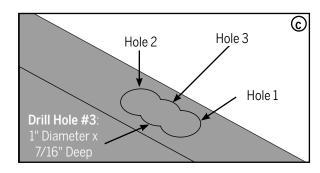
**c.** Drill a third hole directly in between holes 1 and 2. This hole will be 1" in diameter and 7/16" deep.
