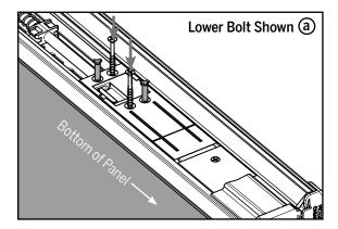
**a.** Keeping the orange securing pins in place, install  $\#8 \times 1-1/2$ " screws in the holes adjacent to the pins.
