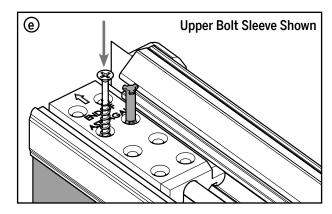
**e.** Install a #8 x 1-1/2" screw next to the popped orange securing pin on the upper bolt sleeve.
