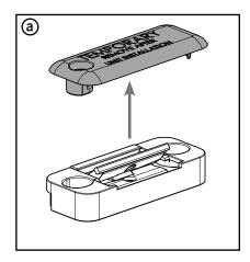
a. Remove the spacer from the keeper assembly.
