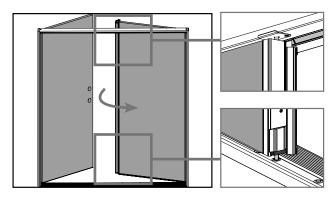
**a.** Close inactive door panel and engage both the upper and lower bolts to ensure they fit into the bolt receivers smoothly.
