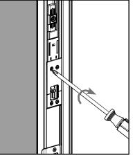
**d.** Tighten the four screws on the deadbolt actuator. **Do not overtighten.**
