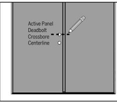
**a.** Determine the deadbolt crossbore centerline of the active door panel and mark this location on the inactive door.
