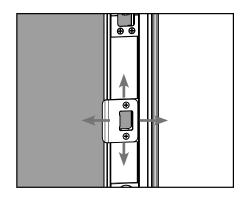
**c.** If the deadbolt actuator is not aligned, return to Step 4. If the strike plate is not aligned, loosen the screws and slightly adjust the location of the plate.
