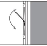
**a.** Close the inactive door panel until the weatherstrip on the header is compressed.
