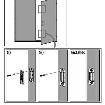
**e.** If the trim strip was removed, reinstall the trim strip so it is flush between the upper lock pawl housing and the deadbolt actuator. If necessary, cut off any excess trim strip.
