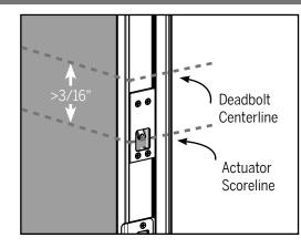
**b.** Check the alignment of the deadbolt actuator with the deadbolt crossbore centerline. If it is misaligned by more than 3/16", adjust the location of the deadbolt actuator as detailed in Step 5. If they are aligned, skip to Step 6.
