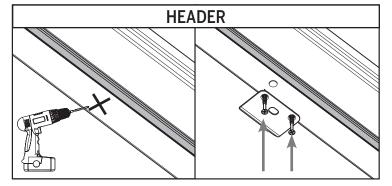
**c.** At the marked location on the header, drill a hole **3/8" in diameter** and at least **1-3/8" deep.** Install the header strike plate into the header, using two #8 x 3" screws.
