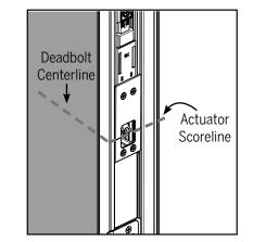
**c.** Adjust the location of the deadbolt actuator so the actuator scoreline aligns with the deadbolt crossbore centerline.
