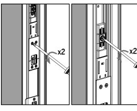
**b.** Loosen the four screws on the deadbolt actuator and actuator adjuster screw two turns each.
