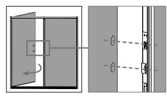
**b.** Close the active door panel and ensure the deadbolt actuator and strike plate are aligned with the crossbore holes in the active door panel.
