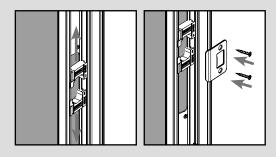
**d.** Adjust the location of the two pieces of the retainer and install the new hardware.
