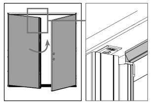
**c.** Close the inactive door panel and ensure the weatherstrip forms a secure seal around the trim cap.
