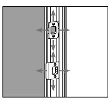
**c.** If it is not aligned, loosen screws and slightly adjust the locations of the plates.
