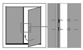
**b.** Close the active door panel ensure the deadbolt and strike plates are aligned with the crossbores on the active panel.
