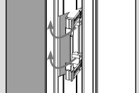
**c.** Break retainer in half using the bend lines. Return the two pieces of the retainer to the astragal and adjust to fit the larger hardware.
