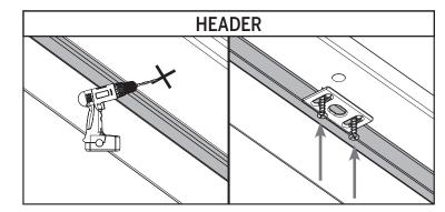
**c.** At the marked location on the header, drill a hole **3/8" in diameter** and at least **1-3/8" deep.** Install the upper strike plate by screwing into the header.
