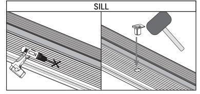
**d.** At the marked location on the sill, drill a hole **5/8" in diameter** and at least **1-3/8" deep.** Install the lower bolt receiver by tapping into the sill with rubber mallet.
