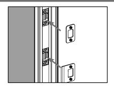
**b.** Install the new hardware into the retainers by tightening the screws through the holes in the plates.
