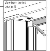
**a.** Close the inactive door. Make a mark at the location where the trim cap contacts the weatherstrip.
