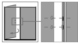
**b.** Close the active door panel and ensure the deadbolt and strike plates are aligned with the crossbore holes in the active door panel.
