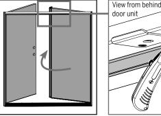
**b.** Open the inactive door. Using a utility knife, make a slit in the weatherstrip along the mark made.
