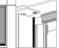
**c.** Close the inactive door panel. Ensure the weatherstrip forms a secure seal around the trim cap.
