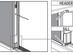
**b.** Press and engage the upper and lower bolts so the bolt pins come in contact with the header and the sill. Mark these points of contact.
