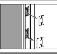
**a.** If installing new strike and deadbolt plates, remove the screws securing the old plates.
