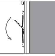
**b.** Engage the flip lever so the upper and lower bolt pins come in contact with the header and the sill. Mark these points of contact.
