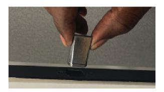
Lift latch away from lock, rotate 180 degrees, place back into lock.
