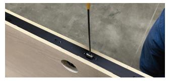
Tighten screw to secure latch in place.
