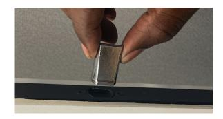
Lift latch away from lock, rotate 180 degrees, place back into lock.
