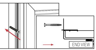
Install fasteners into the upper, middle, and lower prenotched locations in the brickmould connector to secure the unit.
