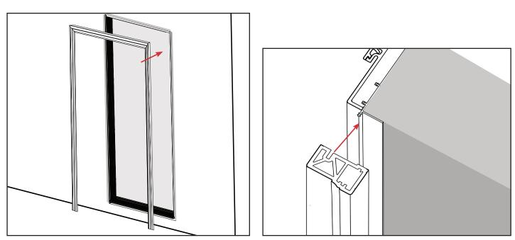
Align the outswing brickmould and re-install the brickmould by pressing firmly to outswing connectors.
