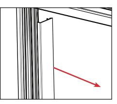
b. Remove the jamb covers using one of the methods outlined below.
