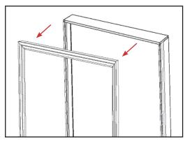
a. If attached, remove the brickmould assembly from the prehung door unit, and set aside.
