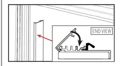
a. Rotate the cover over the jamb (starting from the interior side) and snap it downward along the length of the jamb.
