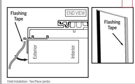
Install flashing tape over the brickmould connector leg as shown.
