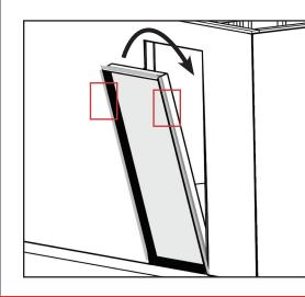
Position the door unit into the rough opening.
