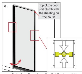
Note: Use a 6' level to confirm that the door unit is aligned properly before securing into place in step 4.
