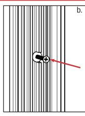
Be sure to insert at least one shim from interior side to keep the jamb from twisting while completing installation..
