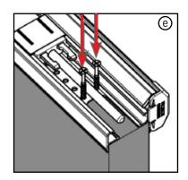
**e.** Install two #8 x 1" screw on the lower most hole next to the U-notch in the astragal body.
