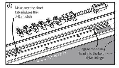
**i.** Return the spine assembly into the astragal, ensuring correct orientation as shown in image below.
