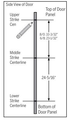
**b.** To determine the middle strike plate centerline, measure 3-5/8" up from the lever crossbore centerline towards the top of the panel and mark.
