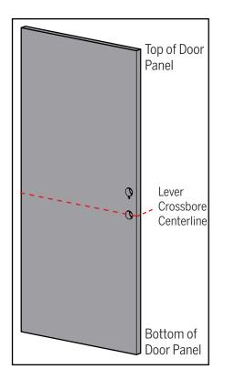
**a**. Determine the inactive door panel's lever crossbore centerline and mark.
