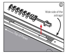
**g.** Remove the spine assembly and set aside to reveal screw holes in the body of the astragal. Remove by lifting from the wide side of the astragal first.
