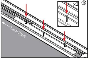
**h.** Install three  $#8 \times 1"$  screws into the astragal body to secure the astragal to the door panel.
