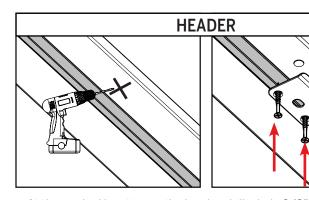
**c.** At the marked location on the header, drill a hole **3/8" in diameter** and at least **1-3/8" deep.** Install one of the strike plates into the header, using two #8 x 3" screws.
