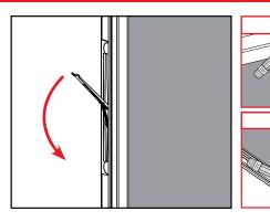
**b.** Engage the flip lever so the upper and lower bolt pins come in contact with the header and the sill. Mark these points of contact.
