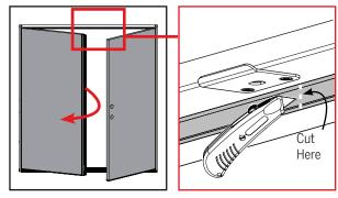
**b.** Open the inactive door. Using a utility knife, make a slit in the weatherstrip along the mark made.
