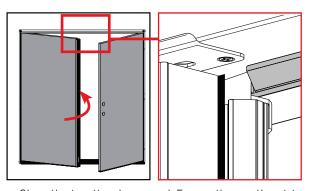
${\bf c.}$  Close the inactive door panel. Ensure the weatherstrip forms a secure seal around the trim cap.
