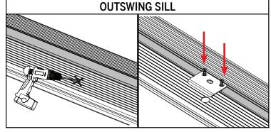
**d.** At the marked location on the sill, drill a hole **5/8" in diameter** and at least **1-3/8" deep.** Install the other strike plate into the sill, using two #8 x 3" screws.
