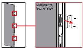
**a.** Remove the upper, middle and lower dummy strike plates.
