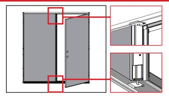
**a.** With the inactive door panel closed, engage both the upper and lower bolts to ensure they fit into the bolt receivers smoothly.
