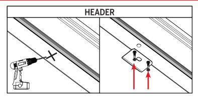
**c.** At the marked location on the header, drill a hole **3/8" in diameter** and at least **1-3/8" deep.** Install the header strike plate into the header, using two #8 x 3" screws.
