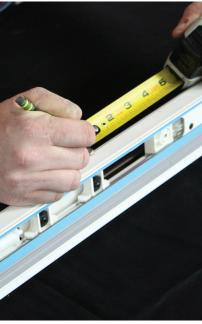
Measure the astragal from the bottom up to the handle height according to your door's specifications. Measure an additional 3 1/2" for the center latch height.
