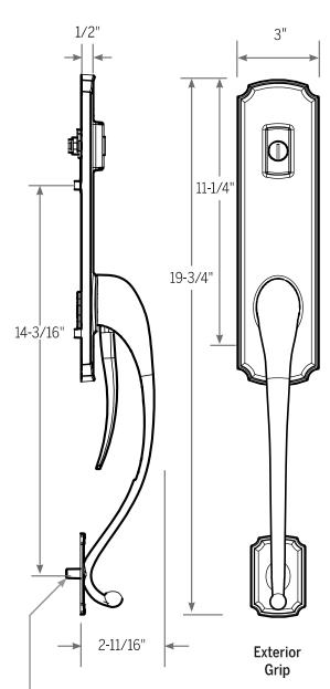
**NOTE**: Drill 3/8" Diameter Hole for bottom of entrance grip mounting screw
