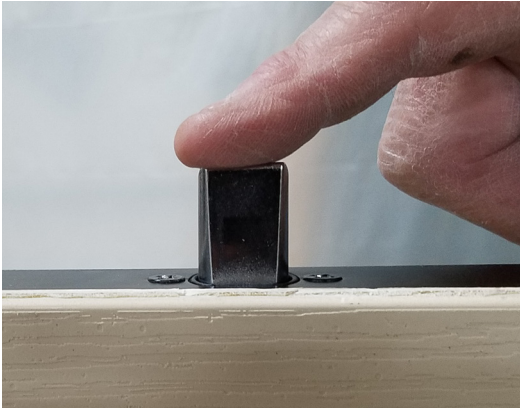
Push down on the center latch. The latch should remain extended.
