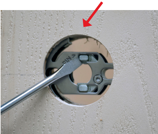
Place a flat head screwdriver next to the pin.
