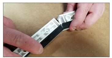
**C.** After cutting through one side the boot can be broken apart.
