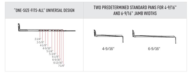
\*Universal design or predetermined standard pans can be sized to fit any opening.
