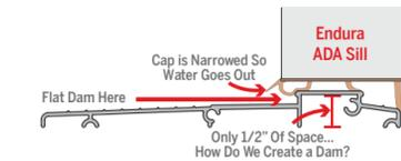
Endura's patented dam feature provides the most effective method for preventing air and water infiltration.
